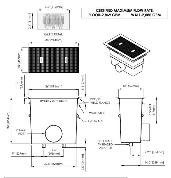
SUMP AND GRATE: UNBLOCKABLE SOFA CERTIFIED TO APSP/ANSI/ICC-16 2017, NSF/ANSI/CAN 50-2020, AND USPC. RPD FIELD CERTIFICATION IS NOT REQUIRED.
